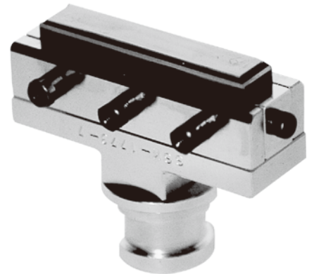
SSK-1000 For Izod Charpy impact test piece 10×80mm JISK-7110-1 K-7111-1
